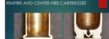
RIMFIRE CARTRIDGE PRIMING COMPOUND IS CONTAINED IN THE INSIDE OF THE RIM OF THE CASE HEAD
